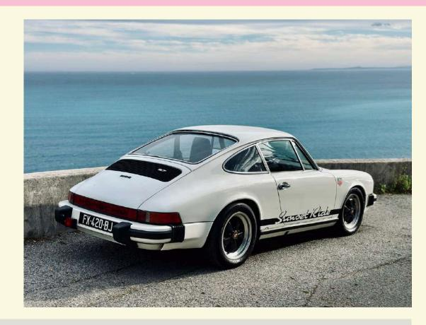
The 1976 Porsche 2.7L G Body is a two-door sports coupe. It is powered by a 2.7-liter flat-six engine, producing 163 horsepower and 173 lb-ft of torque, paired with a four-speed manual transmission. The G Body model features a slightly wider body and improved suspension. It is known for its balanced handling, nimble performance, and engaging driving experience.
