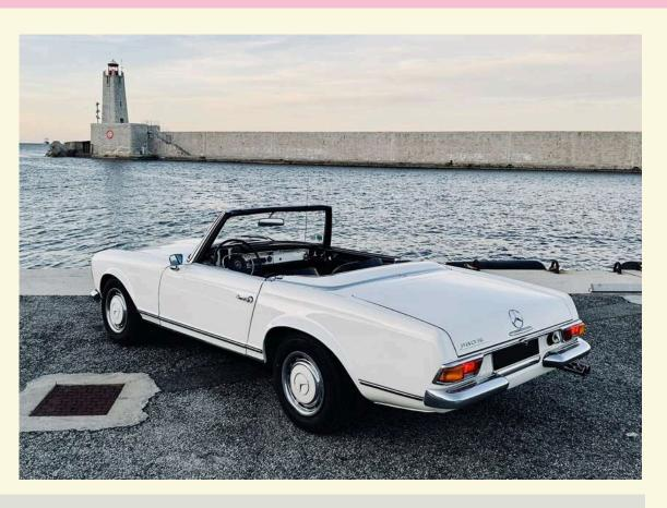
The Mercedes 280 SL Pagoda is a two-seat convertible sports car. The 1970 model is powered by a 2.8-liter inline-six engine, producing 180 horsepower and 177 lb-ft of torque, paired with a four-speed manual transmission. The car is known for its elegant design, smooth ride, and advanced features for its time, such as disc brakes, power steering, and a fully independent suspension.
