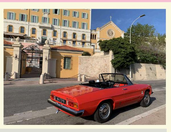
The Alfa Romeo Spider 1300 Junior is a convertible sports car powered by a 1.3-liter inline\( \text{Italian}\) engine, producing 89 horsepower, paired with a five-speed manual transmission. It features classic Italian styling, with sleek lines and a distinctive "shark nose" front end. The car is known for its responsive handling, lively performance, and open-top driving experience
