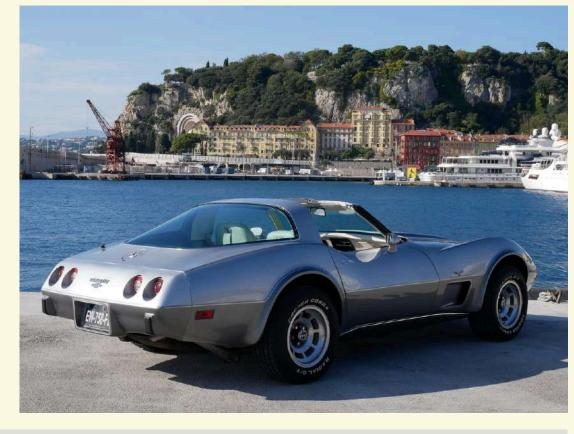
The 1978 Chevrolet Corvette Targa 25th Anniversary Silver Edition is powered by a 5.7-liter V8 engine, producing 185 horsepower and 280 lb-ft of torque, paired with a three-speed automatic. The 25th Anniversary model features a distinctive two-tone silver paint scheme. It is celebrated for its striking design, comfortable ride, and blend of performance with grand touring capabilities.
