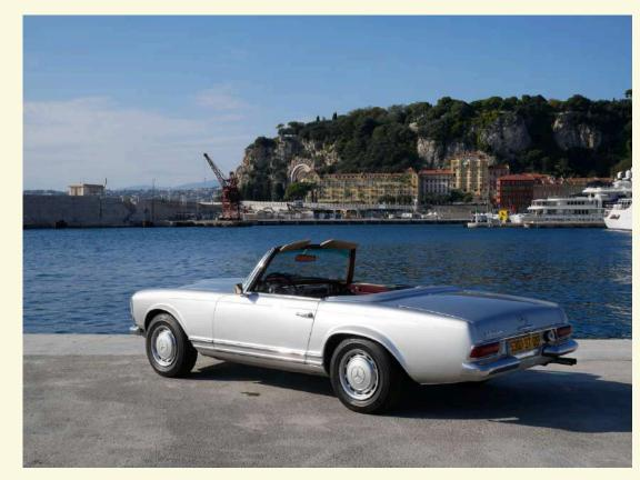
The Mercedes 280 SL Pagoda is a two-seat convertible sports car. This 1968 model is powered by a 2.8-liter inline-six engine, producing 170 horsepower and 177 lb-ft of torque, paired with a four-speed manual transmission. The car is known for its elegant design, smooth ride, and advanced features for its time, such as disc brakes, power steering, and a fully independent suspension.
