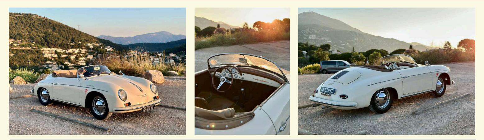
The Porsche 356 Speedster is a two-seat sports car. It features a minimalist design with a low, raked windshield and a removable top. The car is powered by an air-cooled, four-cylinder engine, producing up to 70 horsepower, paired with a manual transmission. The 356 Speedster is known for its nimble handling and performance, making it a favorite among enthusiasts and collectors.
