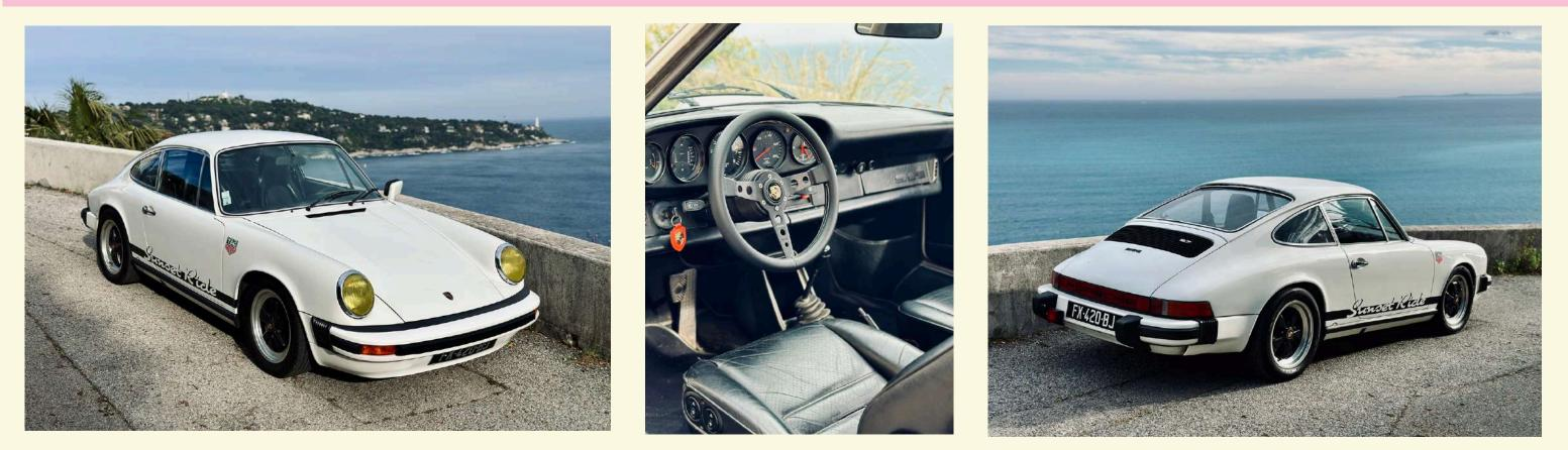
The 1976 Porsche 2.7L G Body is a two-door sports coupe. It is powered by a 2.7-liter flat-six engine, producing 163 horsepower and 173 lb-ft of torque, paired with a four-speed manual transmission. The G Body model features a slightly wider body and improved suspension. It is known for its balanced handling, nimble performance, and engaging driving experience.
