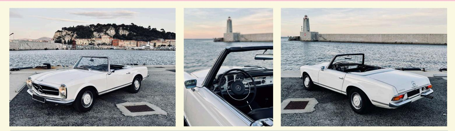
The Mercedes 280 SL Pagoda is a two-seat convertible sports car. The 1970 model is powered by a 2.8-liter inline-six engine, producing 180 horsepower and 177 lb-ft of torque, paired with a four-speed manual transmission. The car is known for its elegant design, smooth ride, and advanced features for its time, such as disc brakes, power steering, and a fully independent suspension.
